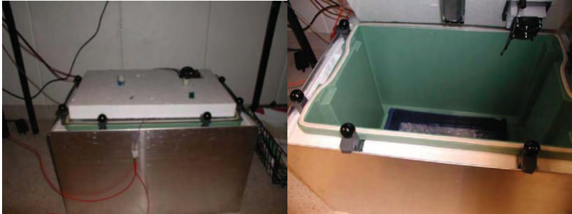
Figure 5: The insulated climate box with circulation fan, thermal regulator and salt solution.
