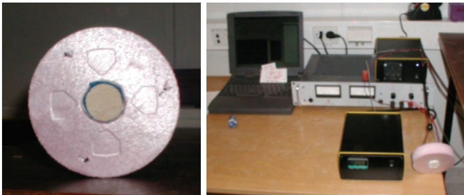
Figure 17: The left image shows the sample holder with a sample in the centre. The right image shows the control units with the sample holder to the right.
