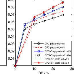
Desorption isotherms at low RH (0-30%) for different binder and different w/b-ratio is very similar.
